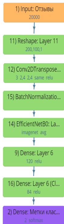
Fig. 3. Modification of the neural network from fig. 2 based on replacing Conv2D with the Conv2DTranspose layer
