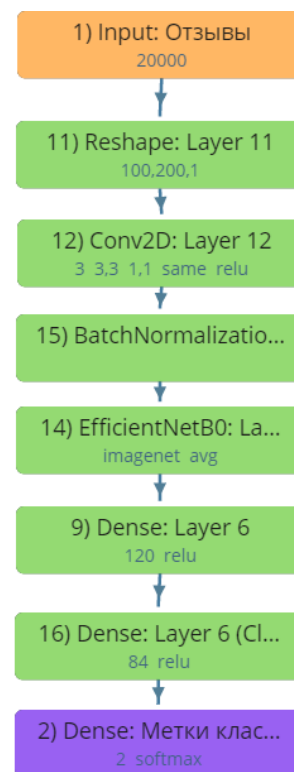
Fig. 2. The proposed neural network for text classification based on the pre-trained EfficientNetB0
